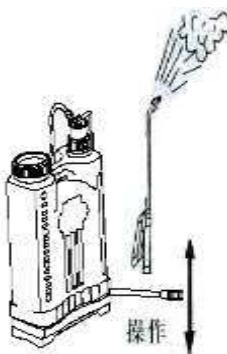
The Spraying parts shall be lubricated after cleaning.
