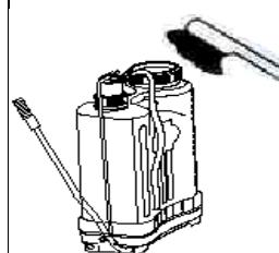
After use, the Sprayer shall be washed to protect it from being eroded by the chemical while avoiding possible chemical reaction between the residual chemical and next chemical when they are of different nature.
